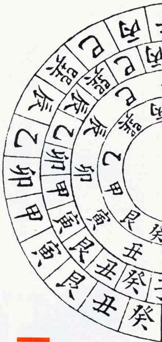
This diagram showing knowledge of the magnetic declination is taken from an early 10th-century geomantic treatise. It is entitled The Directions and Emanations of the Floating Needle , that is, the compass needle floating in a pool of water or mercury.
