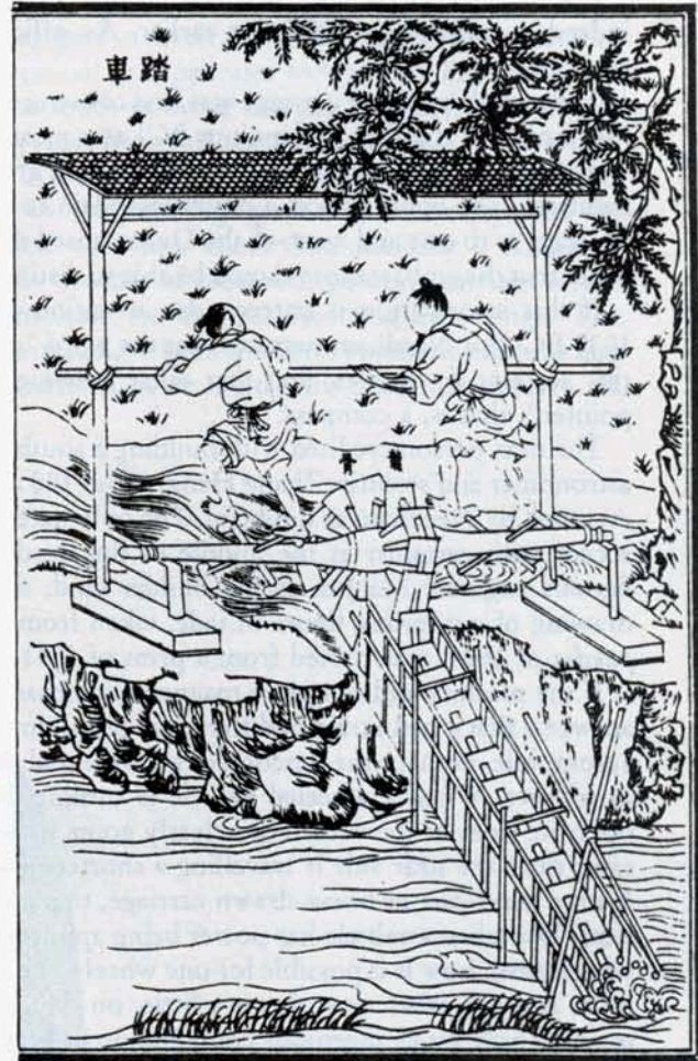
Raising water for irrigation in 17th-century China, using a two-man treadle-operated chain pump.
